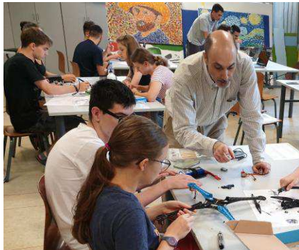
Figure 5 - Students of ICAROS club working on the assembly of drone frames, integration of electronics, testing of components and other tasks to build a complete operational quadrotor drone
